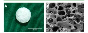
**Figure 1.** Macroscopic (A) and scanning electron microscopy (B) images of demineralized cancellous bone (DCB). (A) Scale bar represents 10 mm; (B) scanning electron microscopy of scaffold at  $\times$ 50, and scale bar represents 500  $\mu$ m.
